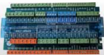
Control Panel Connection Card
