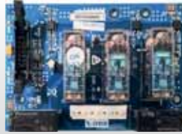
Door Bridging Board
